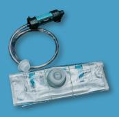
The Puribag Pro is an all-encompassing portable water filtration and treatment system. In 30 minutes or less, the Puribag Pro combines flocculation, sorption, chlorine disinfection, and carbon / HFM filtration to dispense clean drinking water wherever you are.
